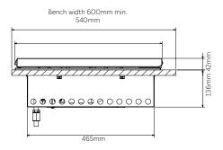
Vent 250mm x 25mm (required when installed separately to barbecue)
