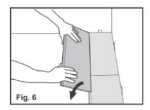
staggered by at least 20". Butt seam (end joint) must be placed in each row regard less of width, e.g. hallways.
