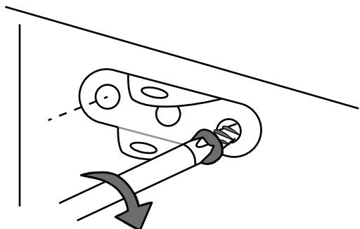
6. Pass the steel wire strap through both mount holes and fasten the connector.
