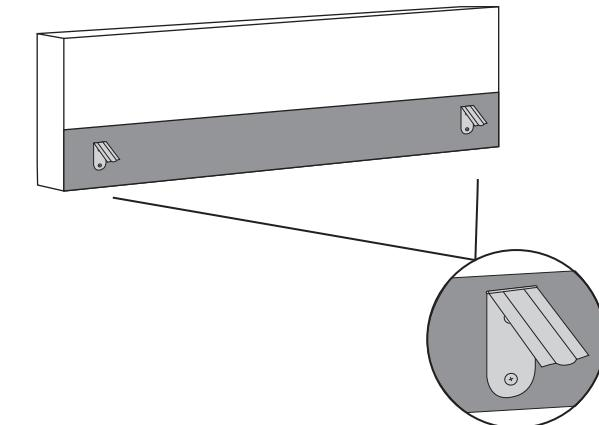
2. Carefully place the backrest, inserting the tabs into the anchors on the structure to secure both pieces.
