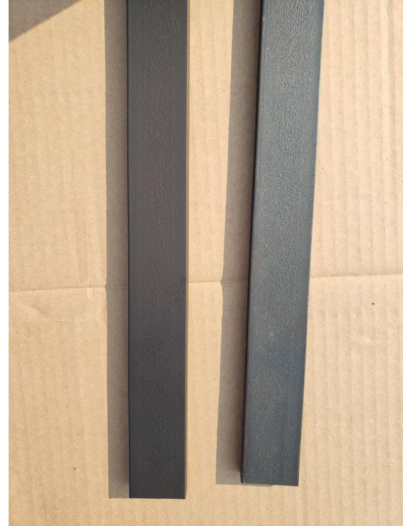
Side by side of clear finish vs. black finish on steel bracket
