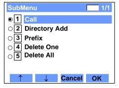
STEP 3: To make a call, select **1 Call** (by using or pressing **1**) and press **(a)**, **(d)** or **OK**.
