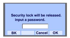
STEP 2: Enter the password and press (Enter) or **OK**. Security Lamp is extinguished and Security Mode is canceled.
