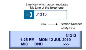
STEP 2: Dial a desired station number. Display indicates the dialed number.
