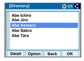
STEP 6: To display the detailed data for a specific name, press Detail while the name is highlighted.
