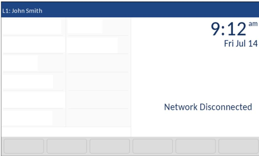
Check that the cables are tightly connected to the phone and to the wall jack. The phone should automatically detect when it is reconnected and remove the Network Disconnected prompt from the screen. However, if changes have been made to your phone's network settings, you may need to restart your phone. Check with your System or Network Administrator for assistance.
