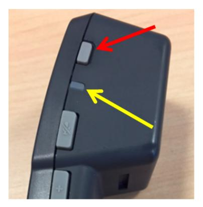
To indicate that the handset is in the pairing mode, the handset LED starts flashing.
