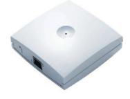
The Spectralink DECT Repeater is a building block used to extend the wireless coverage area within a Spectralink DECT network. The DECT Repeater provides a larger geographical spread of the traffic channels and increases the coverage area. But because it does not increase the number of traffic channels available, the DECT Repeater is mainly used in areas with limited coverage such as long hallways, stairwells and corridors.
