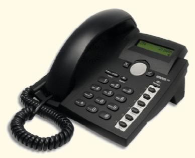
For effective everyday work, the snom 300 provides all relevant office functions such as choice of trunk line, status display, group lines, the engaged option or picking up calls.
