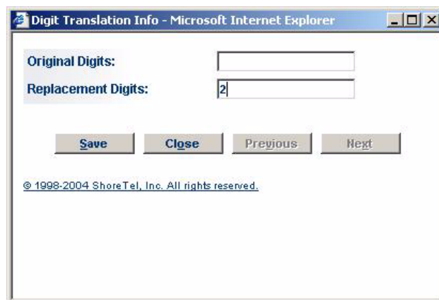
Figure 14-4 Leave Original Digits blank to add a digit to all legacy extensions
