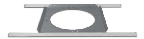
The **SA-TBA** is a tile bridge designed to mount 8 inch loud speaker and bridges both 2 ft x 2 ft and 2 ft x 4 ft ceiling tiles. It is compatible with the Viking models **SA-1S**, **30AE**, **35AE**, **40AE**, **40-IP** and **40TB-IP** ceiling speakers. The **SA-TBA** tile bridge is constructed of 24 gauge cold rolled steel with an electro galvanized rust-resistant finish.
