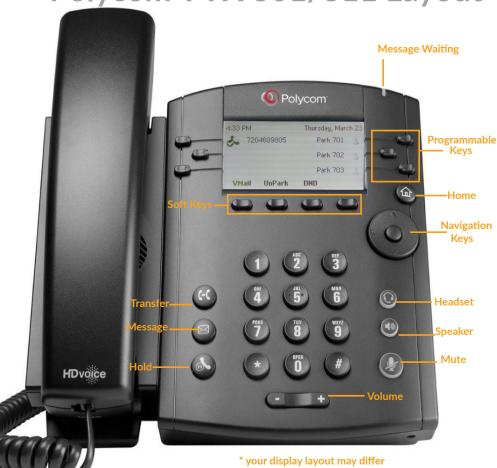
Hold | Press the Hold button or press the Hold soft key. To resume, press the Hold button again or select the Resume soft key. If you have multiple calls on hold, select the call you would like to resume using the navigational keys and perform the second step above.
