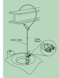
An integral safety cable suspension point on the speaker provides additional safety. A secondary cable can be connected to this suspension point and run alongside the primary (weight-bearing) cable as a backup.
