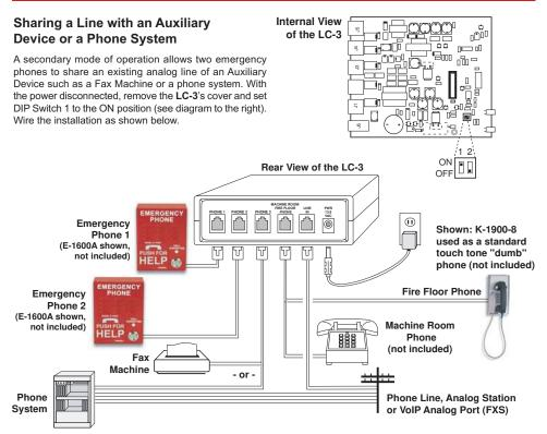
If an emergency phone comes off-hook to place an outbound call while the AUX Device is being used, the phone line is removed to simulate a hang up. After 2 second, fresh dial tone is given to the emergency phone for dialing. Because of this extra delay, it is required that a 4 second pause is programmed at the beginning of each emergency phone's dialing string. The phone system is given a busy signal while an emergency phone call is in place.
