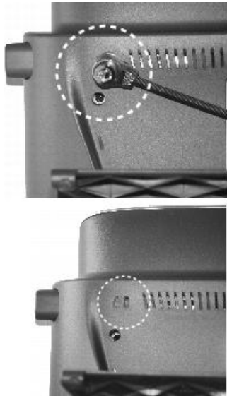
Figure 2: Connecting a Cable Lock to the Cisco Unified IP Phone
