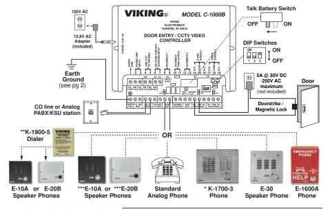
\*\*\* Note: The E-10A and E-20B Speaker Phones may be used without a dialer when installed on a ring-down circuit.
