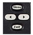
To move forward and back between each feature menu, use the **Arrow** buttons below the **Menu** button. When the feature you want appears, press the softkey below that feature to select it.
