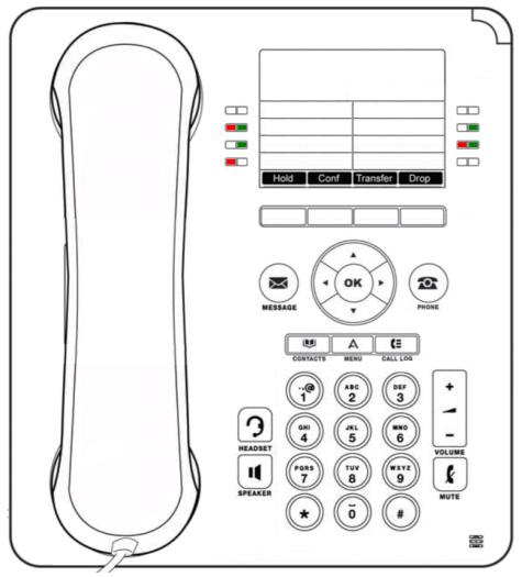
The phone supports 24 programmable call appearance/feature buttons. The labels for these are displayed in the main display and can be controlled by the adjacent buttons.
