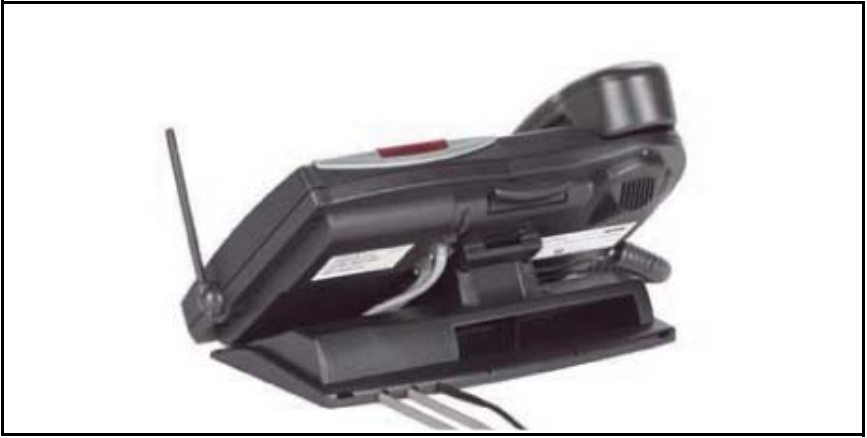
Figure 8: Arranging the cords to exit the stand
