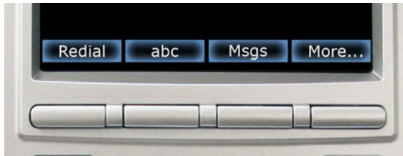
Figure 2: Context-sensitive soft keys when the IP Deskphone is in the idle state
