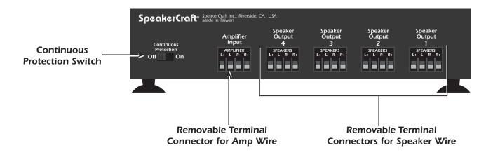
For best results, use speaker wire that is at least 18 gauge. For runs longer than 75 feet, 14 gauge wire is recommended. Wire larger than 14 gauge is not recommended because it may not fit into the connector. For best results, strip all wire insulation no more than 3/8" from the end before inserting into the connector.
