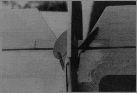
Bottom view of rudder and stab. Shows elevator cross tie and ply control horns.
