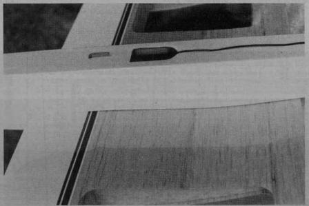
Looking at underside of fuselage at wing location. Shows launching hook and finger hole for hand launching.
