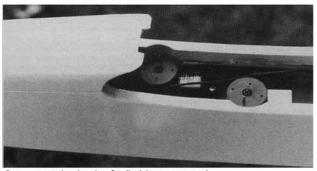
Servos mounted under wing. Small mini servos are used.
