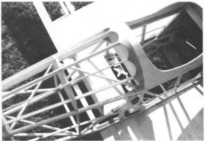
Photo shows location of rudder and elevator servos. They are covered by pilot's seat.
