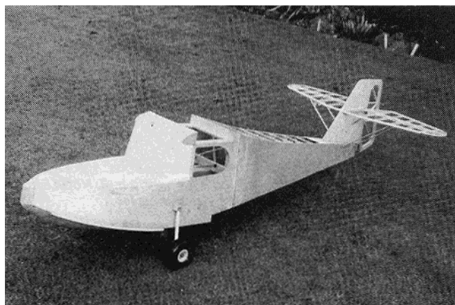
Make windshield pattern from card to establish exact shape.
