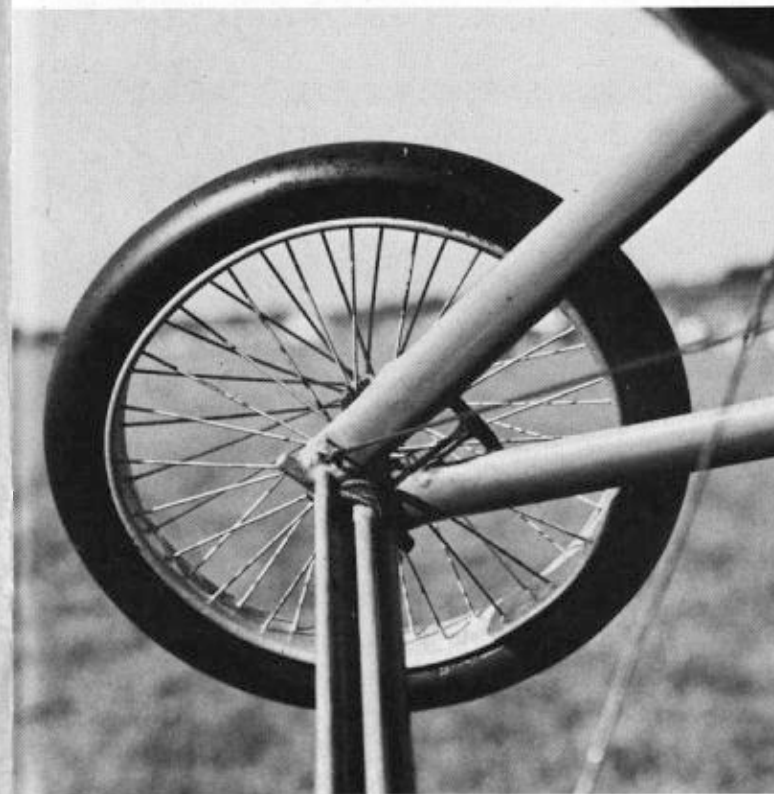
ABOVE: Undercarriage and spring with bungee rubber. BELOW: View of radio installation. Aileron servo, switch access from inside cockpit. Servo access through belly hatch.
