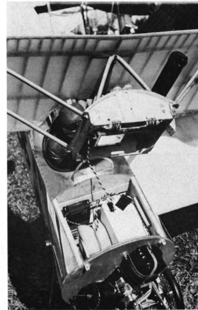
ABOVE: Undercarriage and spring with bungee rubber. BELOW: View of radio installation. Aileron servo, switch access from inside cockpit. Servo access through belly hatch.
