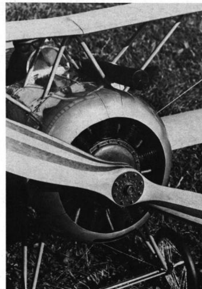
Propeller positioned to cover carburetor. Dummy engine made from balsa, string, cardboard and plenty of filler.
