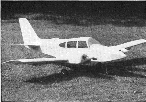
Cougar complete and ready to be covered.
