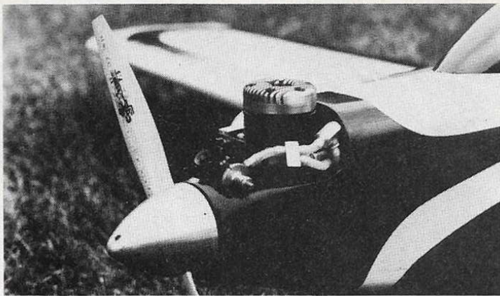
The HP .61 Gold Cup is not only good looking, it's a real powerhouse. Note the Robart pumper and return valve. The engine needs either pressure or a pump (above). A view of the nose's bottom with nosegear doors closed could
