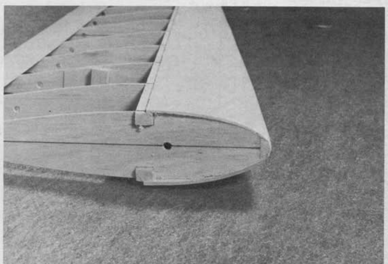
The bottom L.E. sheeting installed and L.E. sanded to shape.
