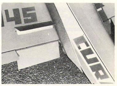
Above: spoilers and flaps. Flaps shown left: partially depressed before the actuation of the spoilers which lift (right) as the flaps reach the extent of their travel. Full detail now added to APS Plan.
