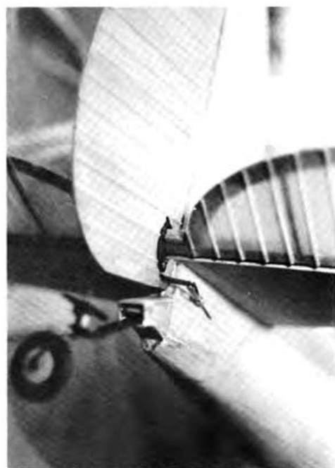
Control horns are formica. Tailwheel springs and chain hook to rudder horn.
