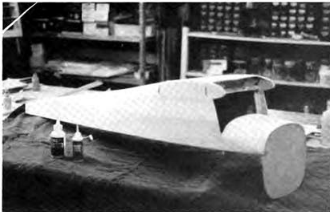
Complete top half of fuselage. Wings and tail should have already been fitted and aligned.
