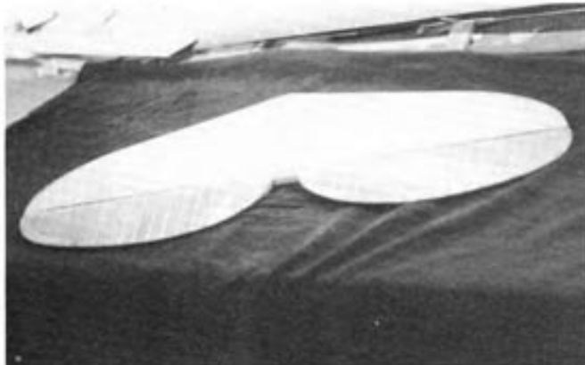
Stabilizer and elevators complete and ready to cover. Balsa sheeted stabilizer is covered with silkspan.
