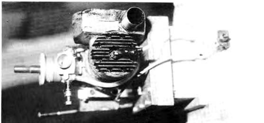
Looking at the bottom of the nose, you can see the extension wires for the glow plug. That's a mini-alligator clip and an old glow plug.
