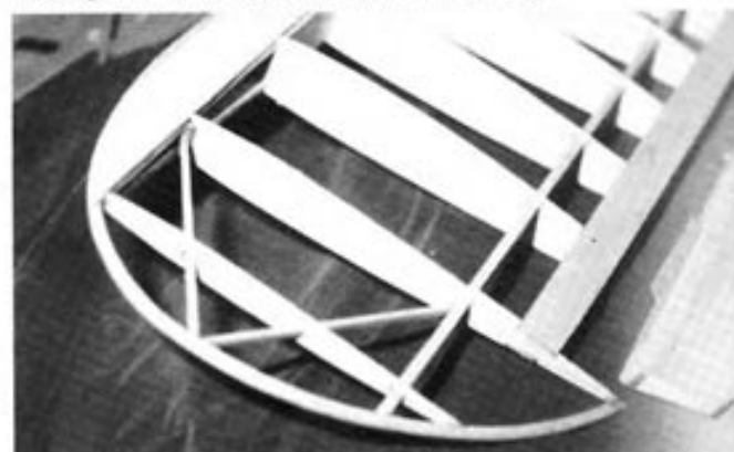
Laminated wing tip is braced with spruce (in case you stand your Cessna on the wing tip while servicing model).
