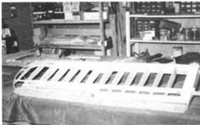
Complete wing with aileron and flaps. Hinges are made up to look scale.
