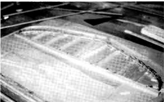
Stabilizer with 1/8 sq. sub-leading edge in place.
