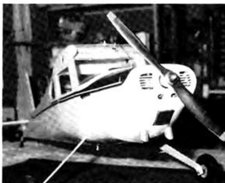
Here is the front end all together, along with the scale prop. The prop is finished with automobile chrome bumper paint; it takes a long time to dry. The dunce cap spinner is molded plastic. Cowl mount screws are counter sunk, socket head screws.
