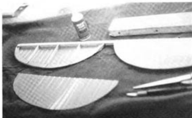
Elevator with most of ribbed plastic installed.
