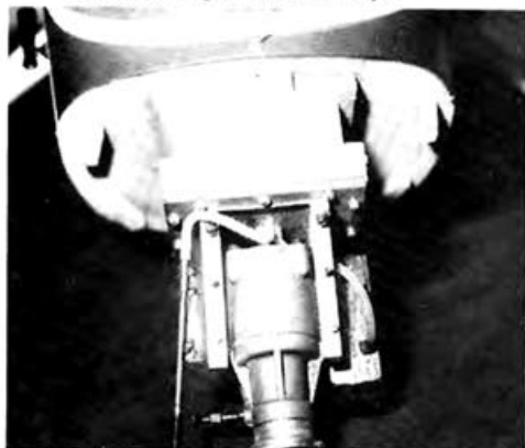
Top view of nose shows cowl and support blocks, fuel fill probe, and general layout. O.S. 1.08 2-stroke engine.
