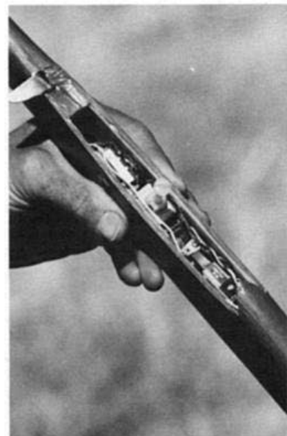
Close-up shot with wing removed shows Rx mounted for easy access to crystal. No case on switch or Rx. Subminiature Futaba S-20 servos used; anything bigger is a no-no. Check Cannon's mini. Photo by Al Kindrick.
