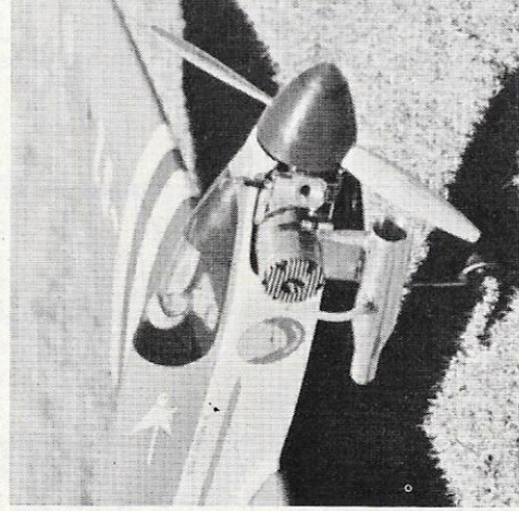
Webra Speed provides the motivation, while Silencaire muffler keeps things legal and quiet.
