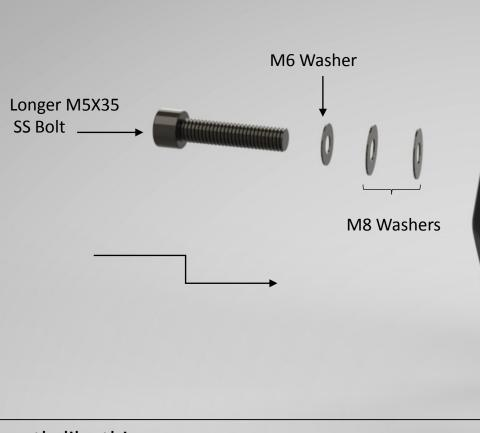
Complete assembly goes on the bike's top mounting hole
