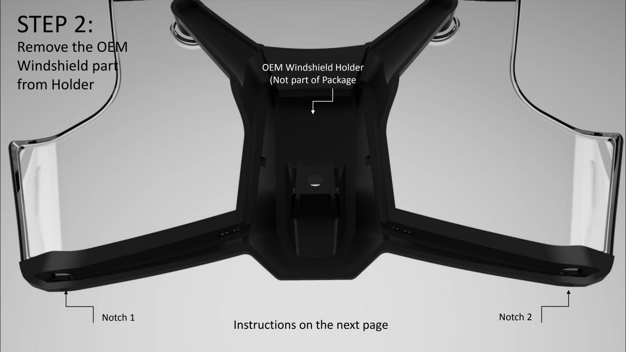
Carefully press the Notches on each side of the holder which are holding the windshield in place. Use the smallest Screw Driver you can find. Make sure that you don't rush this step. Any excess force may break the clear part as it is acrylic.
