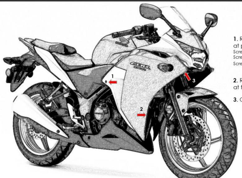
1. Remove the 4mm Allen key screws at points 1, 2 and 3.
