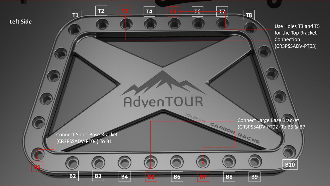
Step 3: Connect Side Brackets to the Bike Wheel Arch Bolts
