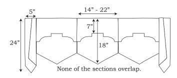
A tail can be placed at each end of the valance sections. **The tail is 5" wide and about 24" deep** from the top of the pole. It does not have a return, which makes it important to use decorative brackets to install the pole. The depth of the tail can be altered. It attaches to the top of the pole with hook and loop tape, or staples.
