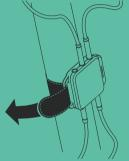
Simply wrap the strap around the tripod leg and slide the strap into the slot. Once through, pull tight and securely fasten the strap back to itself.
