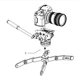
Mount the tripod head/camera over StandONE by rotating it clock-wise. If you are using a tripod head with a 3/8"-16 mounting port, you will need to attach the included adapter screw(1).
