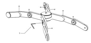
You can adjust the tension of the system with the help of a 3mm allen wrench (1). Simply tighten or loosen the screws as shown above.
