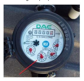
5. And the circle gauge at the left is the hundredths of a gallon pumped.
