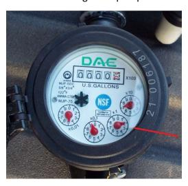
4. The circle gauge at the bottom is the Tenths of a gallon pumped.
