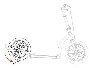
When you're ready, fold the kickstand down with the legs closed as shown above.
