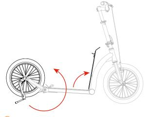
Lift the footplate and rotate the rear wheel.
