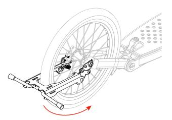
Using your toe to pivot the kickstand down to the ground, roll the scooter backwards until the kickstand snaps into place underneath the rear wheel.
