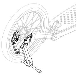
The final standing position, the rear wheel is lifted, with the stand underneath.
