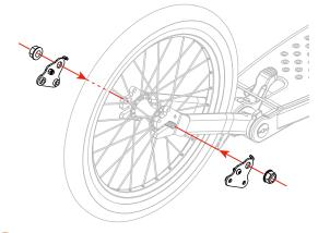
Attach the two retaining plates to the axle and secure them in place using the wheel nut. Please note the orientation as shown above.
