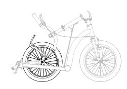
The kickstand will rotate through the frame into the fully folded position as shown above.
