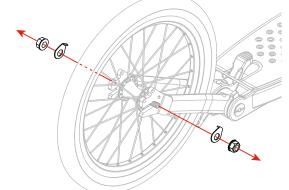
Remove wheel nuts and retaining washers. Set aside the retaining washers and keep in a safe place.
