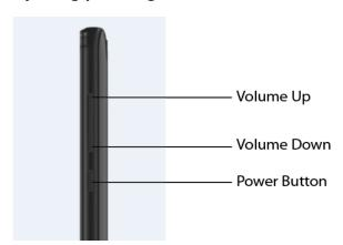
Alternatively, you can also press the volume-up or down button, located on the top-right side edge of your device (with the screen facing you).
