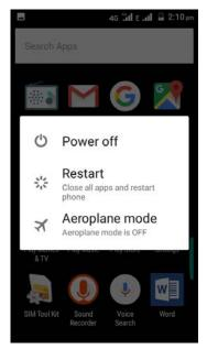
**Turn off the phone:** Tap 'Power off' to turn the phone off. Alternatively, you can press power button for more than 5 seconds.
