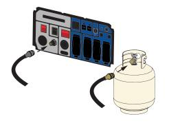
Step 1: Connect the included propane line to the generator and to the propane tank.
