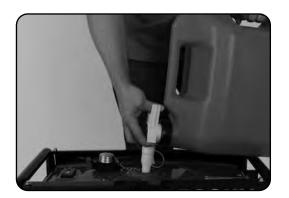
If you have been using gasoline in your generator; before storing your generator for extended periods of time you should drain your generator fuel tank of gasoline.
