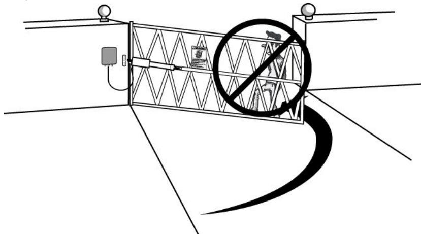
8. Pedestrians should never cross the pathway of a moving gate. The gate opener is not acceptable for use on any pedestrian gate. Pedestrians must be supplied with a separate pedestrian access.
