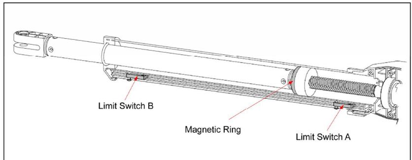
**NOTE:** Always place the magnetic ring between the Limit Switch A and B.
