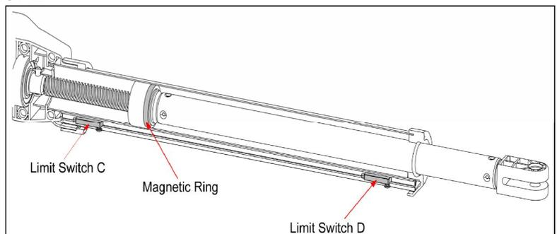
**NOTE:** Always place the magnetic ring between the Limit Switch C and D.
