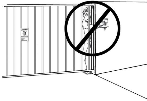
11. Controls intended to be used to reset an operator after 2 sequential activations of the entrapment protection device or devices must be located in the line of sight of the gate, or easily accessible controls shall have a security feature to prevent unauthorized use. Never allow anyone to hang on or ride the gate during the entire travel of the gate.
