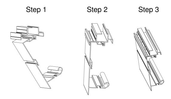
We recommend you permanently attach the Base sections to the Floor Profiles with Self Tapping metal screws – 3 screws in front and back and 5 screws on each side.
