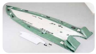
Begin by folding the extensions in half. Keep folding toward the valves and pushing air out.
