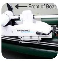
Place motor over Quick Release plate and insert locking bar. Locking bar must engage the clip. Follow manufacturer's instructions for deploying and stowing the motor. For Watersnake, see the next page of this manual.
