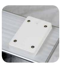
Attach Quick Release adapter block to aluminum board using M6 x 40 mm (1 ½") socket head screws, washers and locking nuts. The sides are tapered, install so that block and base can slide together.
