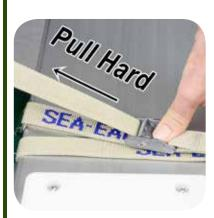
Run strap end through buckle. Hold buckle open with one hand, pull on free end with other hand. Pull tight, check inside loop, make sure it's pulled tight.
