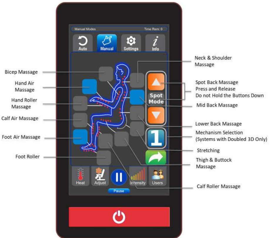
Fig.11: Manual Control Screen
