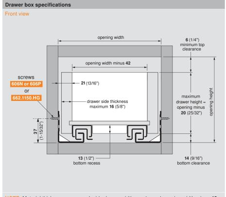
NOTE: Material thickness may vary. Inside drawer width must equal opening width minus 42 for TANDEM to align and function properly.
