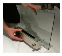
Place and thread each thumb screw (with vinyl washer) through the glass and base, and then tighten securely, DO NOT OVER TIGHTEN as you may break the glass.
